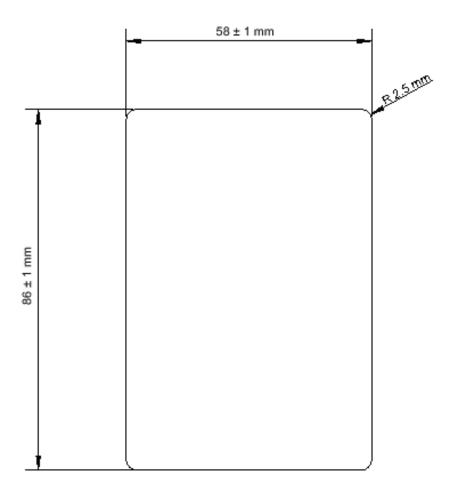
Figure 1-3 Door mounting kit drilling pattern
