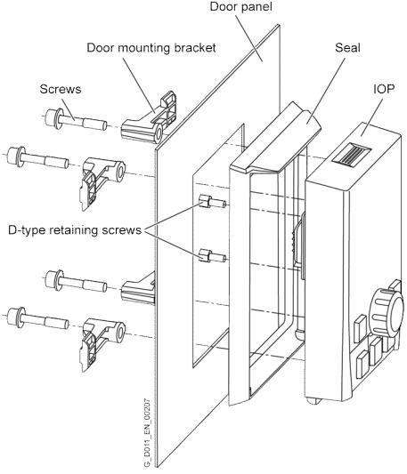
Figure 1-1 Installation of IOP door mounting kit
