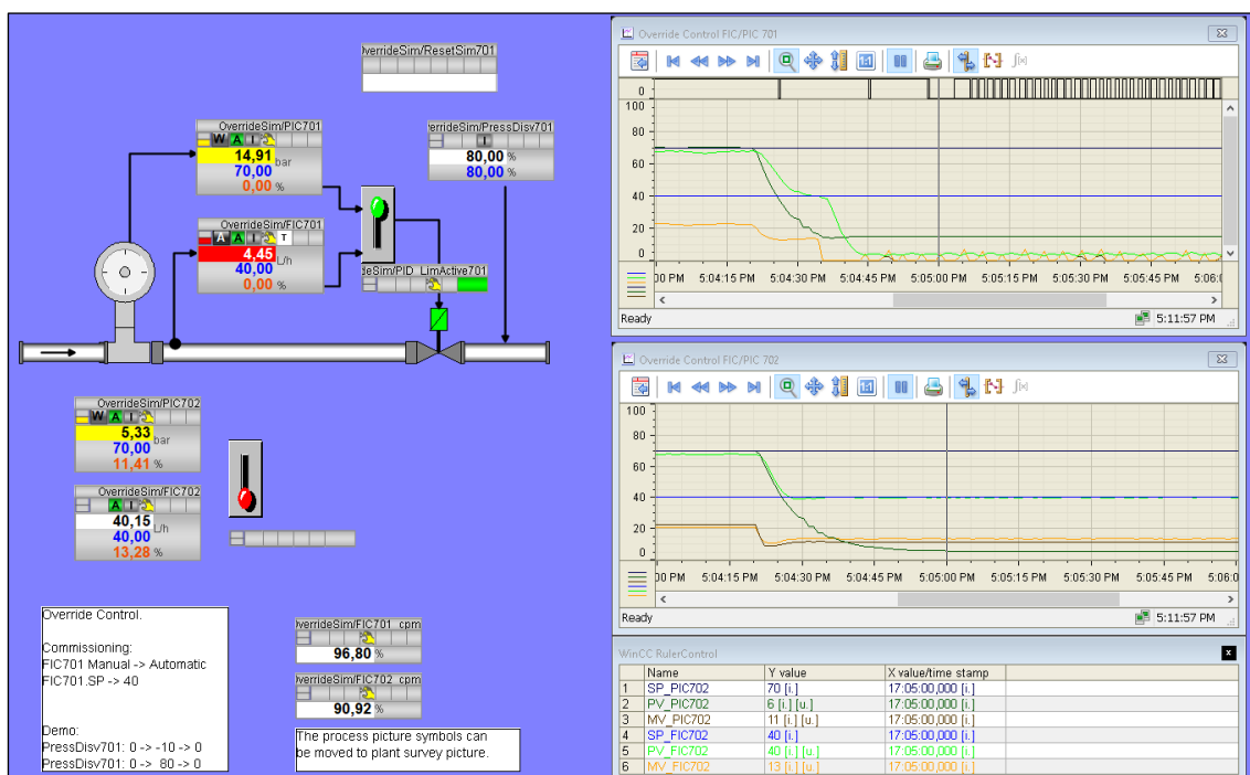
Figure 4-4 Behavior of the override control scheme for a decrease of pressure (after approx. 5:04h)
