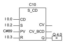
A change in signal state from 0 to 1 at input I0.2 sets counter C10 with the value 89. If the signal state of input I0.0 changes from 0 to 1, the value of counter C10 is decreased by 1, unless the value of counter C10 is equal to 0. The signal state of output Q4.0 is 1 if counter C10 is not equal to 0. If I0.3 changes from 0 to 1, the value of C10 is set to 0.
