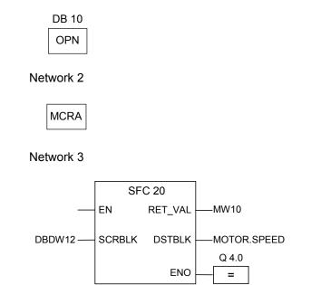
The networks shown above are program sections of a function block created by the user. DB10 is opened in this block and the MCR activated. If the unconditional SFC20 call is executed, the following happens:
