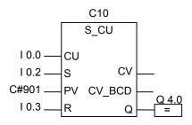
A change in signal state from 0 to 1 at input I0.2 sets counter C10 with the value 901. If the signal state of I0.0 changes from 0 to 1, the value of counter C10 is incremented by 1, unless the value of C10 is equal to 999. If I0.3 changes from 0 to 1, the value of C10 is set to 0. The signal state of output Q4.0 is 1 if C10 is not equal to 0.
