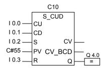
A change in signal state from 0 to 1 at input I0.2 sets counter C10 with the value 55. If the signal state of input I0.0 changes from 0 to 1, the value of counter C10 is incremented by 1, except when the value of counter C10 is already 999. If input I0.1 changes from 0 to 1, counter C10 is decremented by 1, except when the value of counter C10 is already 0. If I0.3 changes from 0 to 1, the value of C10 is set to 0. Q4.0 is 1, when C 10 is not equal to 0.
