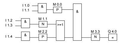
The edge memory bit M3.3 stores the signal state of the previous RLO.
