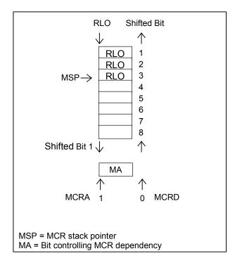
The MCR< instruction adopts the signal state of the RLO and copies it to the MCR bit.
