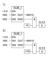
If the signal state at input I0.0 is 1, the SUB\_I box is activated. If the value of input word IW0 is greater than the value of input word IW2, the result of the math function IW0 - IW2 is greater than 0. If the signal state of EN is 1 (activated) and an error occurs while the instruction is being executed, the signal state of ENO is 0.
