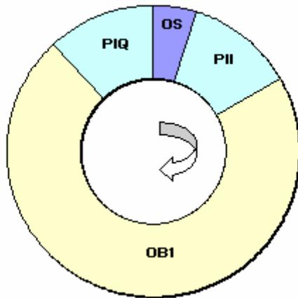
One of the internal tasks of the operating system (OS) is to read the status of inputs into the process image input table (PII). Once this step is complete, the user program is executed with all blocks that are called in it. The cycle ends with writing the process image output table (PIQ) to the outputs for the modules. Reading in the process image input table and writing the process image output table to the outputs for the modules is all independently controlled by the operating system.
