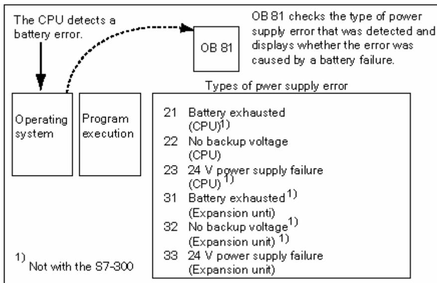
You can write a program that evaluates the event code triggered by the OB81 call. You can also write a program that brings about a reaction, such as activating an output connected to a lamp on the operator station.
