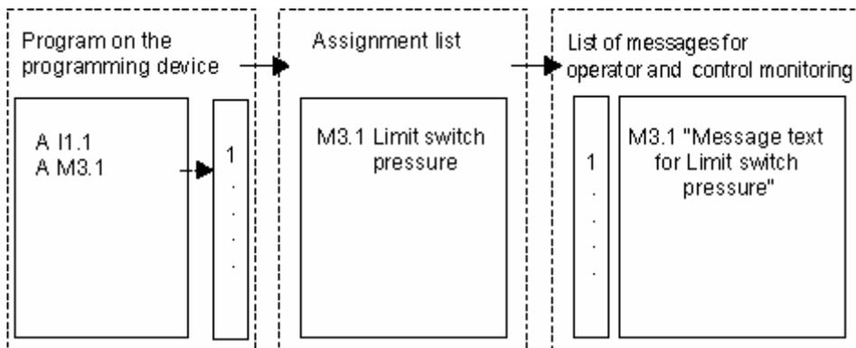
The operator interface system queries the programmable controller cyclically to see whether the message bit has changed or not. If the programmable controller signals a change, the corresponding message is displayed. The message receives the time stamp from the operator interface system.
