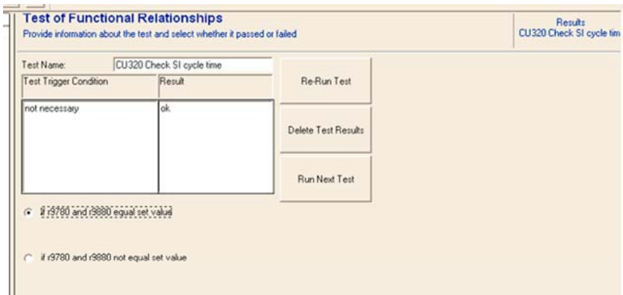
Figure 13-23 Test 2: Checking the SI monitoring clock cycles
