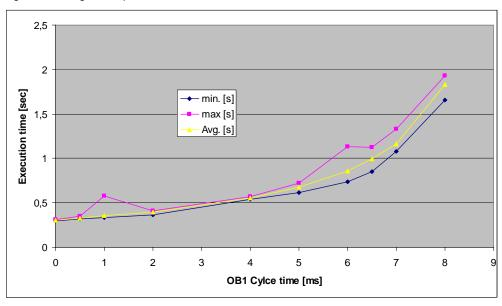
Figure 3-3 Diagram of performance of the AccessDB V2 driver
