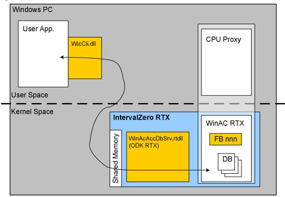
The user application includes (uses) the DLL **WIcCli.dll**. This DLL communicates via Inter Process Communication (IPC) with the WinAC ODK real-time driver **WinAcAccDbSrc.rtdll**.
