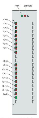
Figure 5-1 LED displays of the DI 16x24VDC HF module
