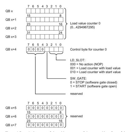
Figure 4-5 Assignment of the address space of the control interface of the DI 16x24VDC Count (bytes 0 to 7)
