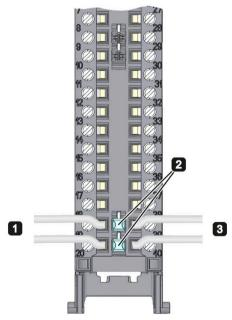
Figure 3-3 Using the potential jumpers
