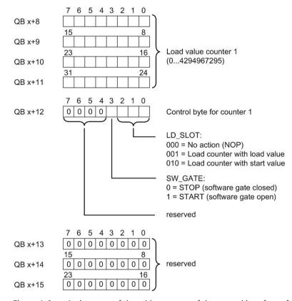
Figure 4-6 Assignment of the address space of the control interface of the DI 16x24VDC Count (bytes 8 to 15)
