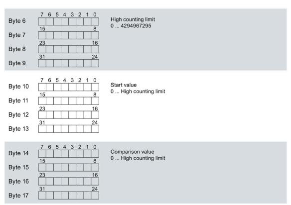
Figure B-3 Structure of data record 0: Bytes 5 to 17
