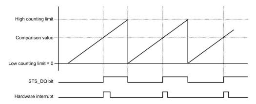
Figure 4-11 Behavior of the STS\_DQ bit and hardware interrupt
