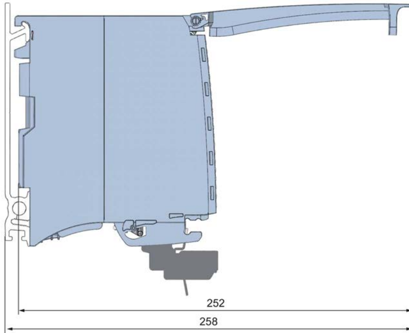
Figure A-2 Dimensional drawing of the TM Count 2x24V module, side view with open front panel
