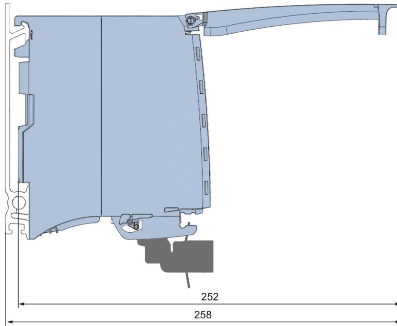
Figure A-2 Dimensional drawing of the AI 8xU/I/RTD/TC ST module, side view with open front panel
