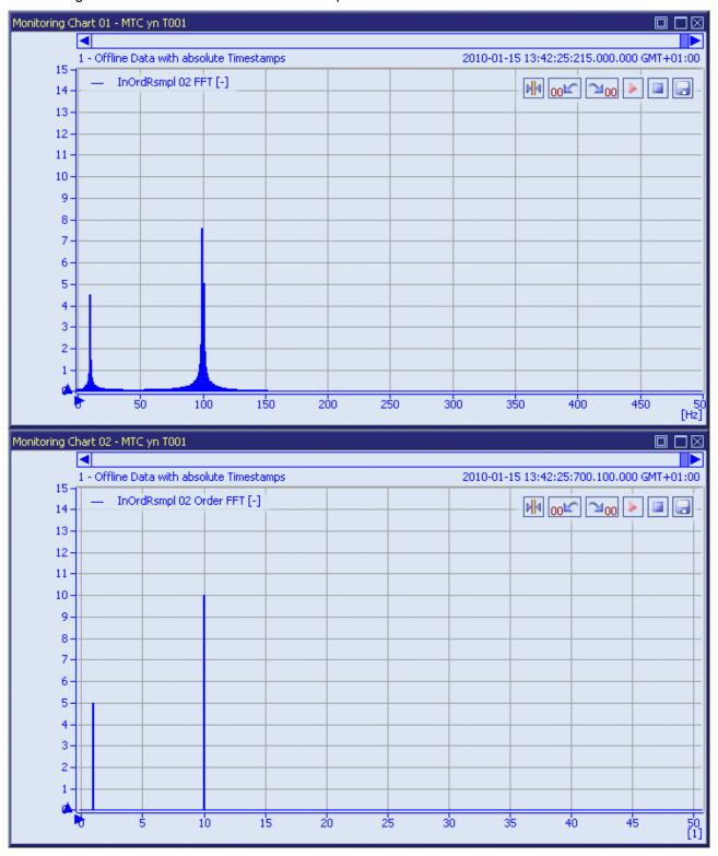
Figure 62: Example of a Frequency Spectrum and of an Order Spectrum
