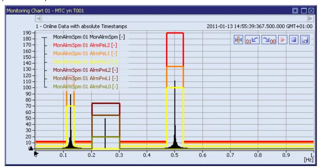
Figure 59: Example of the derived Input Spectrum with Alarm Spectra
