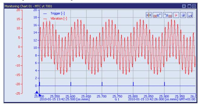
Figure 61: Example of the Input Signals for the Order Analysis
