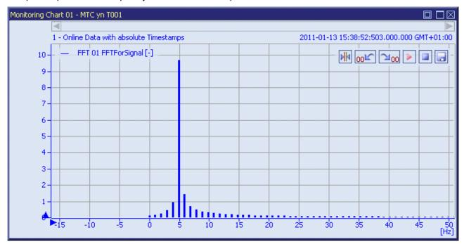
Figure 54: Example of a Frequency Spectrum which has been calculated by the Frequency Analysis
