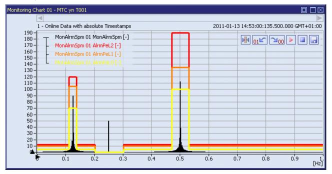
Figure 57: Example of the Input Spectrum with Alarm Spectra
