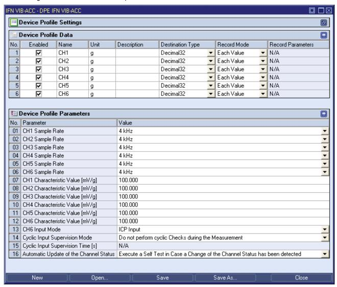
Figure 10: Example of a DPE IFN VIB-ACC
