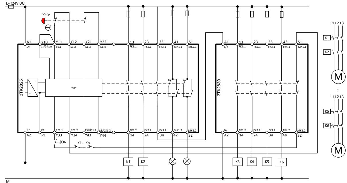
Wiring diagram 3SK1 Standard
