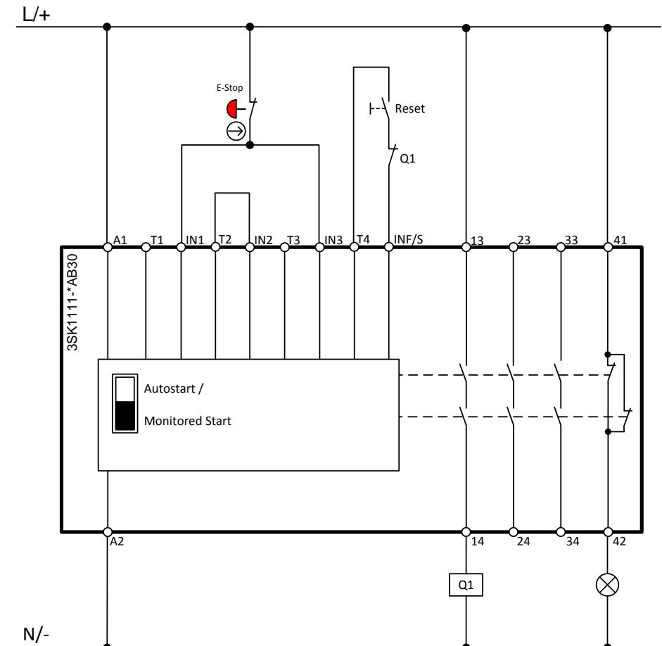
Wiring diagram 3SK1 Advanced
