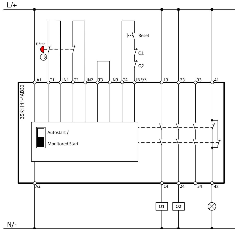
Wiring diagram 3SK1 Advanced
