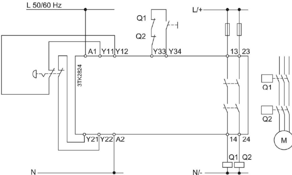
Wiring diagram 3SK1 Standard
