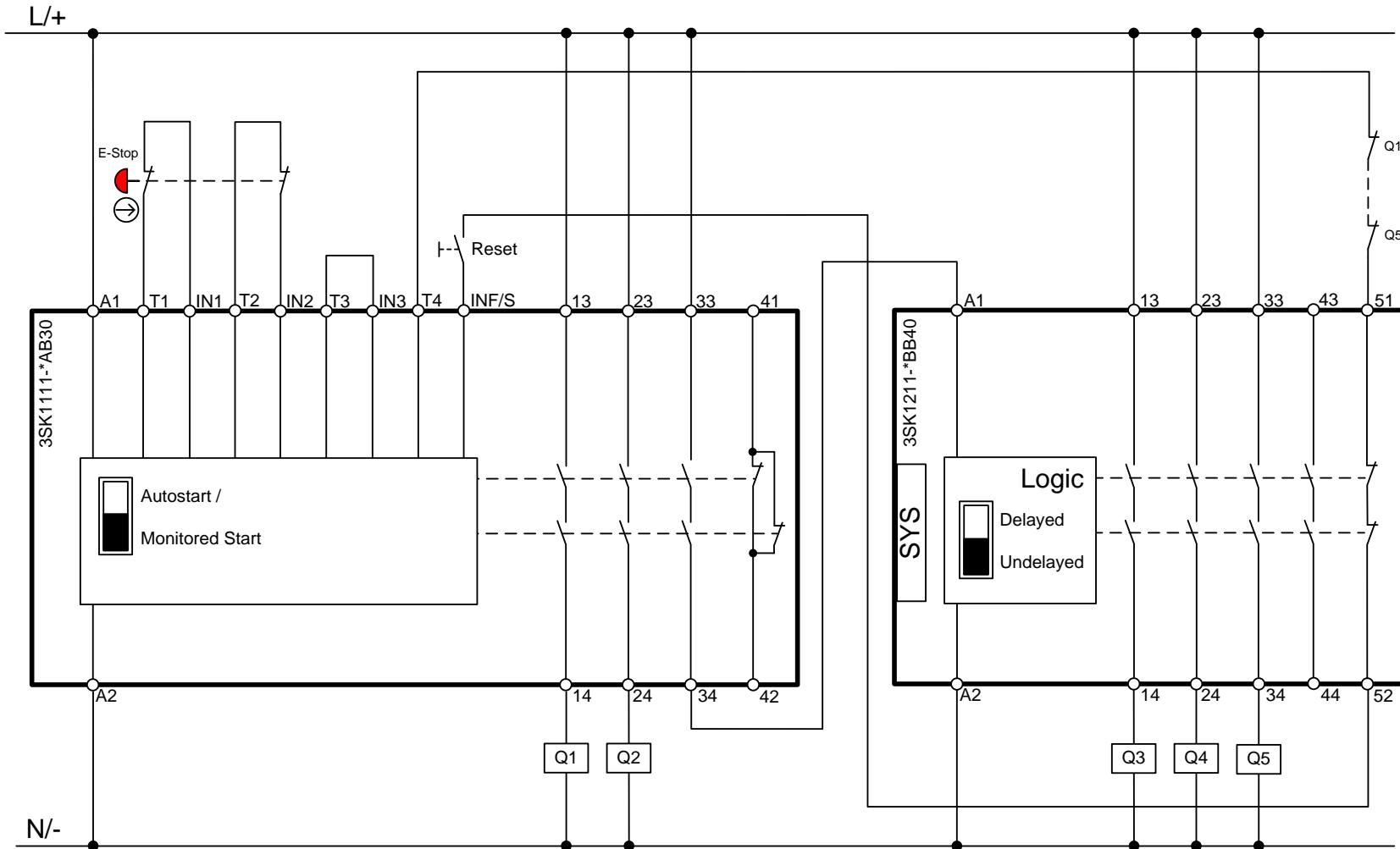
**Wiring diagram 3SK1 Advanced**
