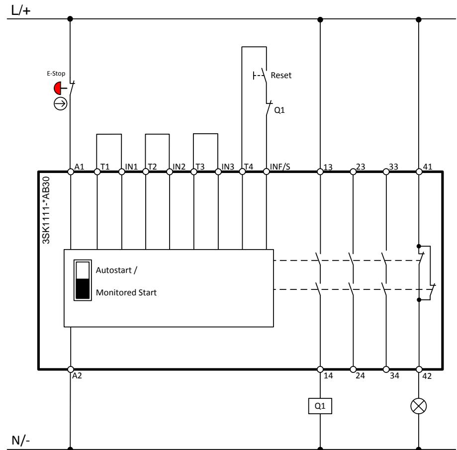
Wiring diagram 3SK1 Advanced
