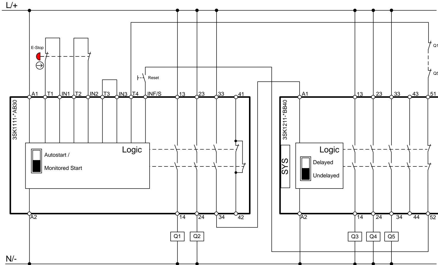
Wiring diagram 3SK1 Advanced
