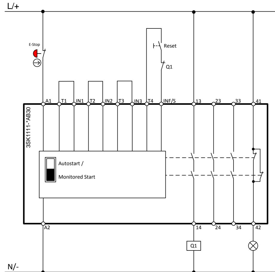
Wiring diagram 3SK1 Advanced
