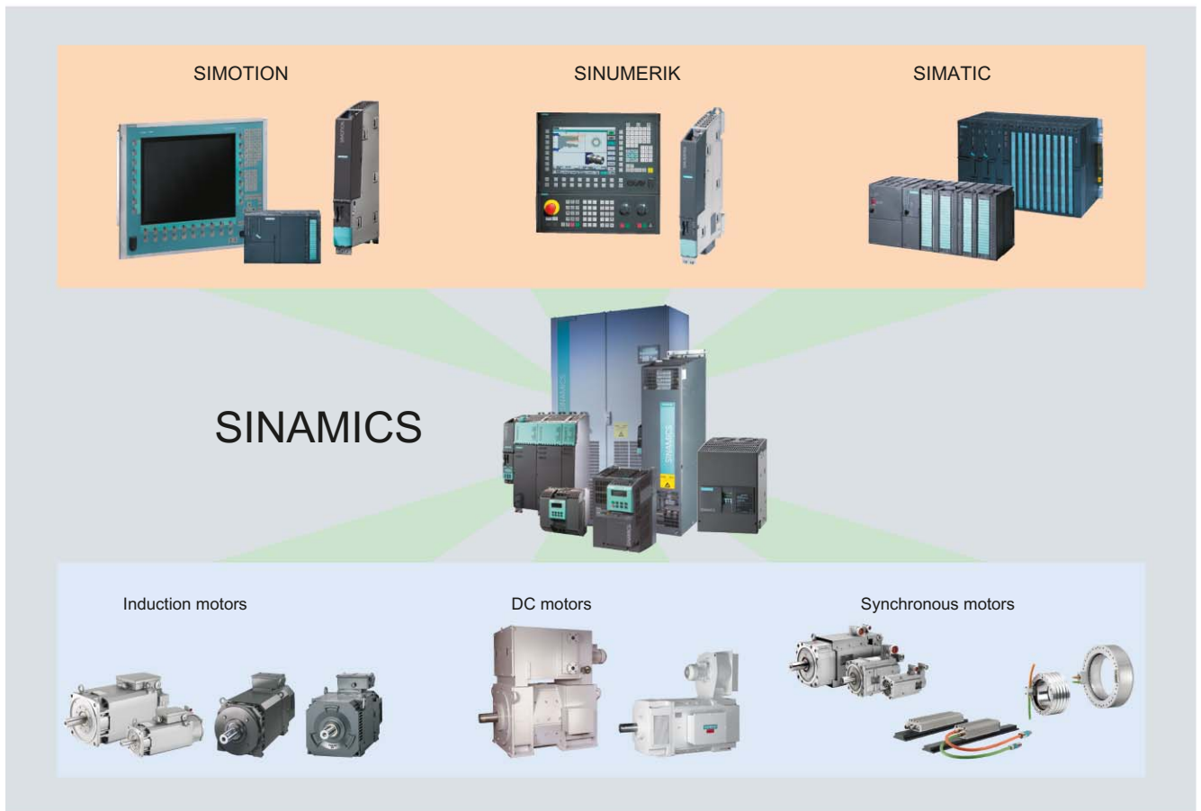
Figure 2-2 SINAMICS as part of the Siemens modular automation system
