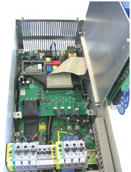
Compact device W=225, connector for external control voltage
