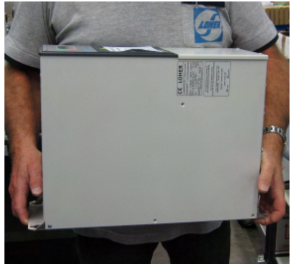
Lifting compact devices - correct
