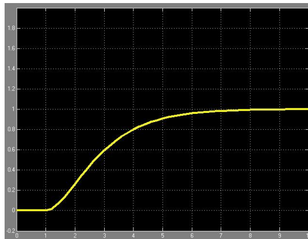
Figure 2-8: Step response of PT2 element with D > 1
