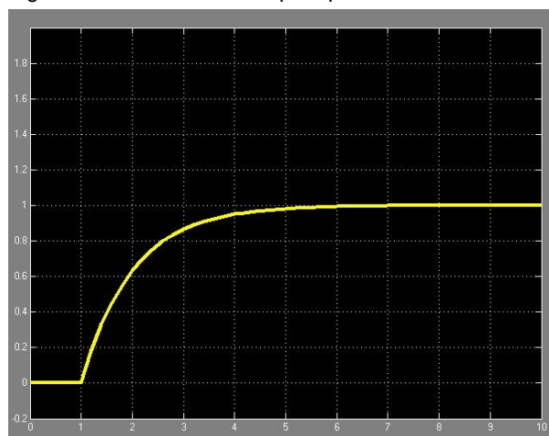
Figure 2-2: PT1 element step response
