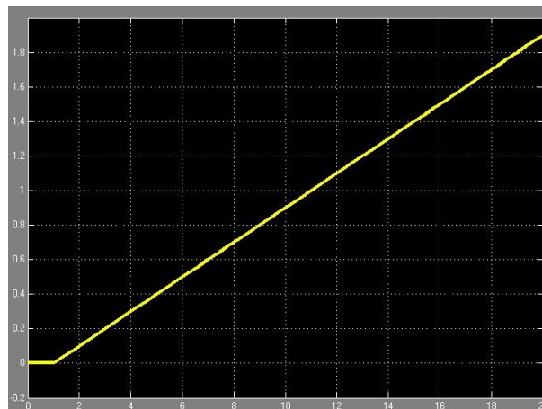
Figure 2-15: I element step response
