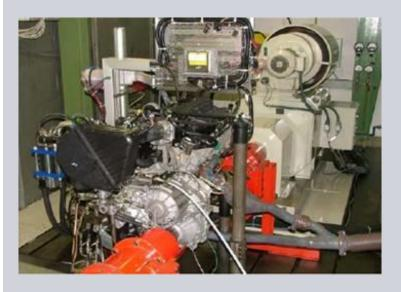
Field test of the CCP on a Ford gearbox with 6RA7085-6DV62-0 and CCP: 6RA7085-6FC00-0
