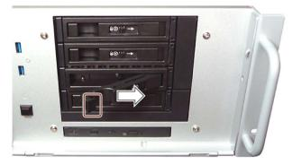
4. Now grip the handle to the right of the notch from where it was pulled out, and pull the tray all the way out of the removable drive bay.
