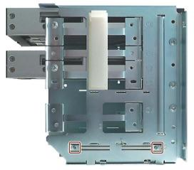
The figure below shows the positions of the screws on the right side of the drive cage.
