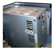
4. Remove the four fixing screws that are marked in the figure below.
