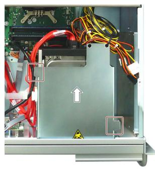
3. Hold the drive cage at the marked areas, push it in the direction of the arrow, then lift the drive cage completely out of the device.
