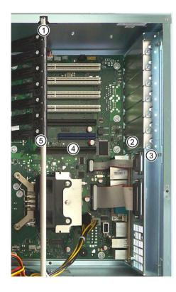
1. Hold the bar ① with the card retainer on both ends and remove it by pulling it upwards.
