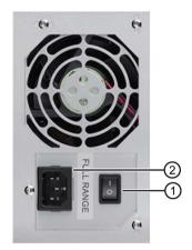
1. Make sure that the on-off switch ① is in the '0 '(off) position.
