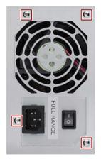
5. Pull the power supply upward and out of the housing.
