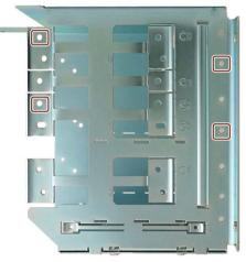
The figure below shows the possible positions of the screws on the right side of the drive cage.
