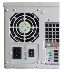
Connect the identified equipotential bonding connection to the protective conductor of the control cabinet in which the device is installed.
