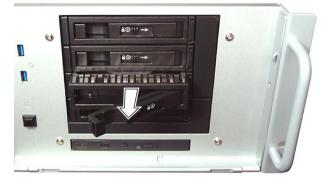
5. Loosen the highlighted screws on the bottom of the tray and remove the drive.
