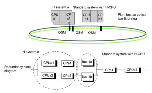
Figure 14-17 Example of redundancy with fault-tolerant system and fault-tolerant CPU
