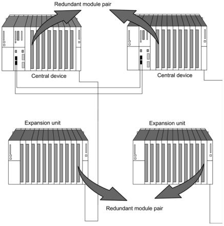
Figure 13-3 Redundant I/O in central and expansion devices
