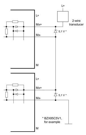
Figure E-31 Interconnection example 2 SM 331; AI 8 x 0/4...20mA HART
