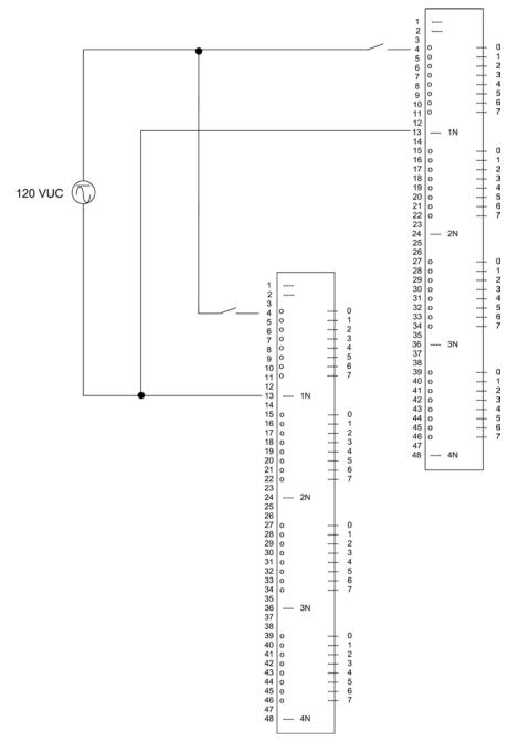
Figure E-10 Example of an interconnection with SM 421; DI 32 x UC 120 V
