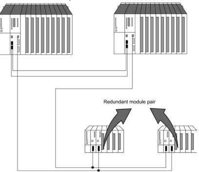
Figure 13-5 Redundant I/O in the switched DP slave
