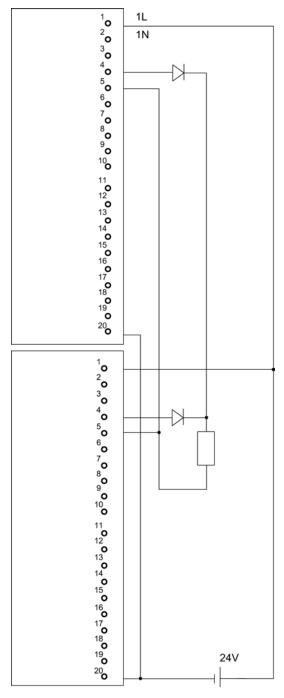
Figure E-22 Example of an interconnection with SM 332; AO 4 x 0/4...20 mA [EEx ib]
