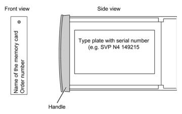
Figure 5-4 Design of the memory card
