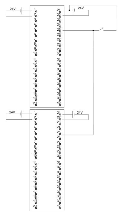
Figure E-9 Example of an interconnection with SM 326; DI 24 x DC 24 V
