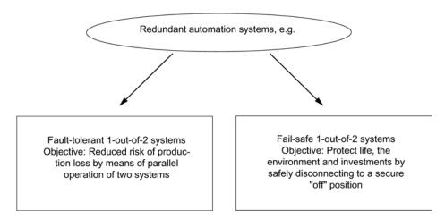
Figure 2-1 Operating objectives of redundant automation systems
