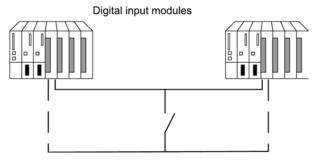
Figure 13-7 Fault-tolerant digital input module in 1-out-of-2 configuration with one encoder
