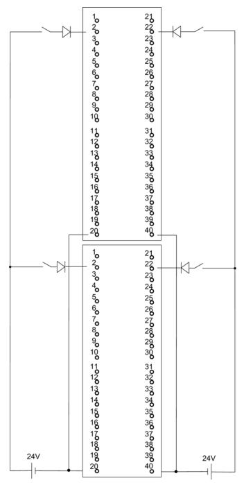
Figure E-2 Example of an interconnection with SM 321; DI 32 x DC 24 V
