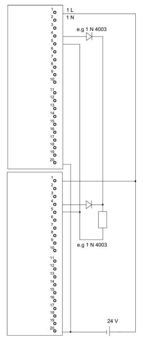
Figure E-17 Example of an interconnection with SM 322; DO 16 x DC 24 V/10 mA [EEx ib]
