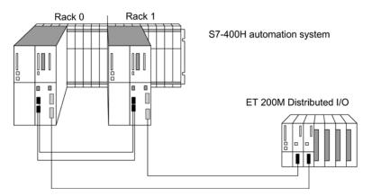
Figure 13-2 Single-channel switched distributed I/O configuration at the PROFINET interface
