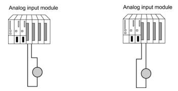
Figure 13-11 Fault-tolerant analog input modules in 1-out-of-2 configuration with two encoders
