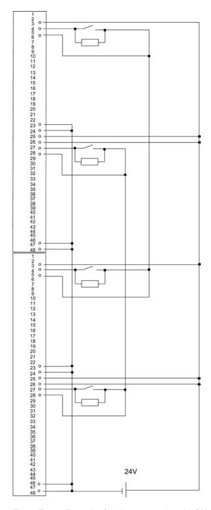
Figure E-11 Example of an interconnection with SM 421; DI 16 x 24 V
