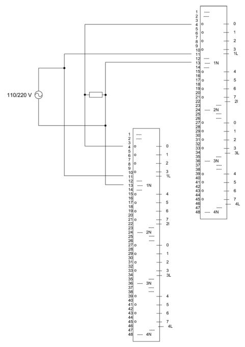
Figure E-23 Example of an interconnection with SM 422; DO 16 x 120/230 V/2 A
