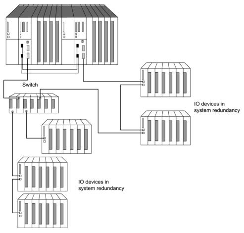
Figure 8-4 PN/IO with system redundancy
