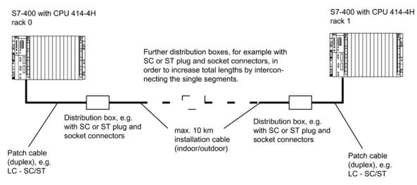
Figure 18-2 Fiber-optic cables, installation using distribution boxes
