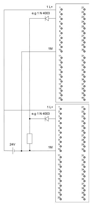
Figure E-15 Example of an interconnection with SM 322; DO 32 x DC 24 V/0.5 A
