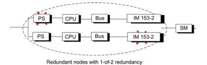
Figure 2-5 Example of redundancy in a 1-out-of-2 system with total failure
