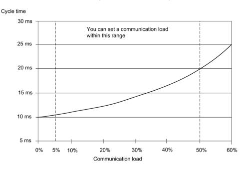
Figure 19-6 Dependency of the cycle time on communication load
