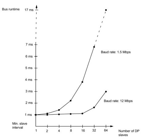
Figure 19-7 DP cycle times on the PROFIBUS DP network
