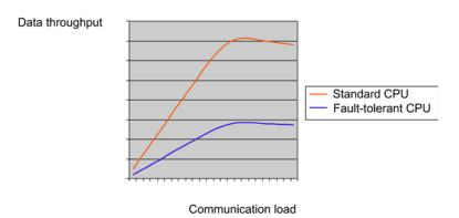
Figure 14-20 Communication load as a variable of data throughput (basic profile)
