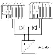
Figure 13-12 Fault-tolerant analog output modules in 1-out-of-2 configuration
