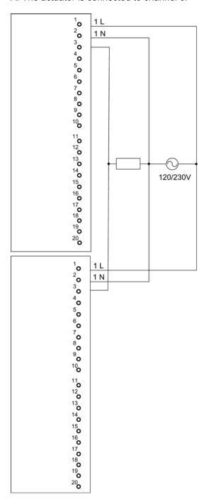
Figure E-16 Example of an interconnection with SM 322; DO 8 x AC 230 V/2 A
