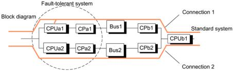
Figure 14-8 Example of linking standard and fault-tolerant systems in a redundant bus system
