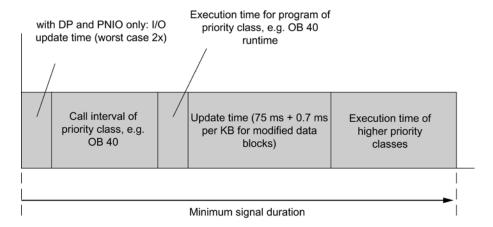
Figure 12-3 Example of minimum signal duration of an input signal during the update
