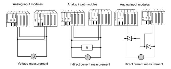
Figure 13-10 Fault-tolerant analog input modules in 1-out-of-2 configuration with one encoder
