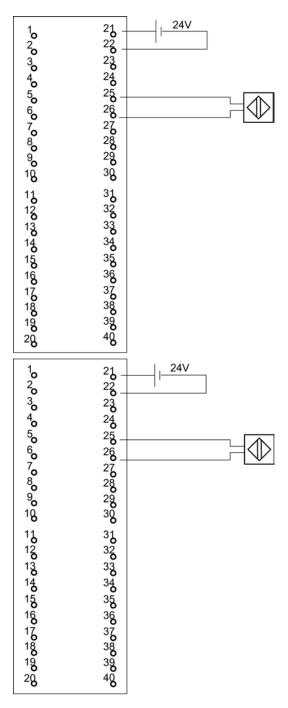
Figure E-8 Example of an interconnection with SM 326; DI 8 x NAMUR
