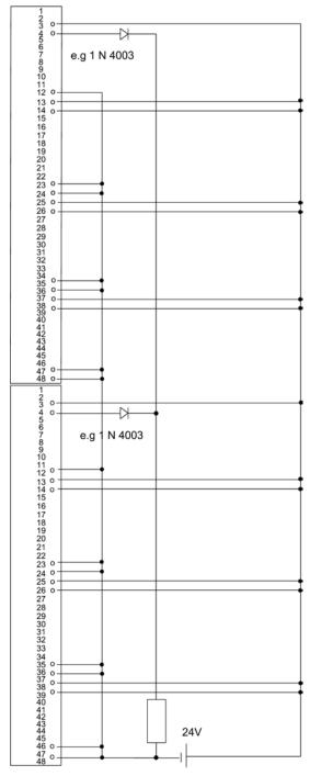
Figure E-24 Example of an interconnection with SM 422; DO 32 x DC 24 V/0.5 A
