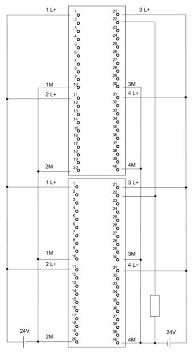
Figure E-20 Example of an interconnection with SM 322; DO 16 x DC 24 V/0.5 A
