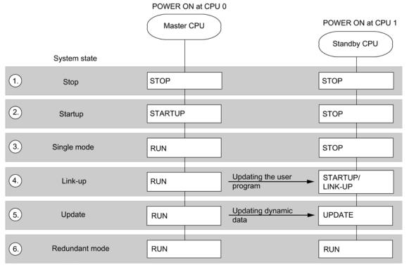
Figure 11-2 System and operating states of the fault-tolerant system
