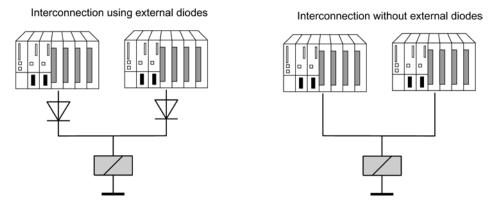
Figure 13-9 Fault-tolerant digital output modules in 1-out-of-2 configuration
