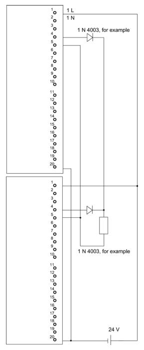
Figure E-18 Example of an interconnection with SM 322; DO 16 x DC 15 V/20 mA [EEx ib]
