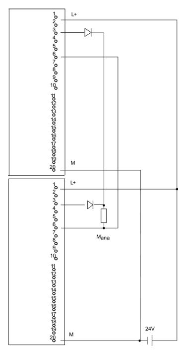
Figure E-32 Example of an interconnection with SM 332, AO 4 x 12 Bit
