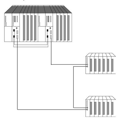
Figure 8-2 S7-400H system with IO devices connected in system redundancy
