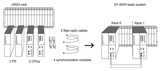
Figure 3-2 Hardware of the S7–400H basic system
