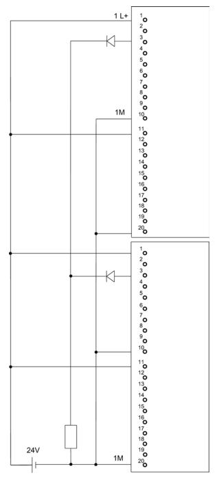
Figure E-14 Example of an interconnection with SM 322; DO 8 x DC 24 V/2 A
