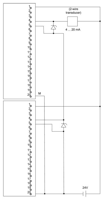
Figure E-25 Example of an interconnection with SM 331, Al 4 x 15 Bit [EEx ib]
