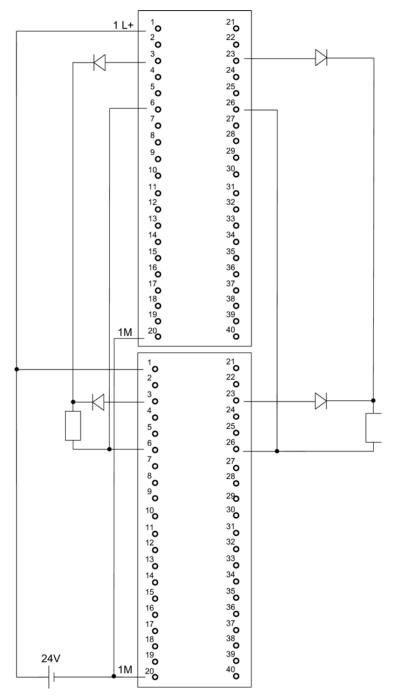
Figure E-21 Example of an interconnection with SM 332, AO 8 x 12 Bit
