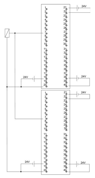
Figure E-7 Example of an interconnection with SM 326; DO 10 x DC 24V/2A
