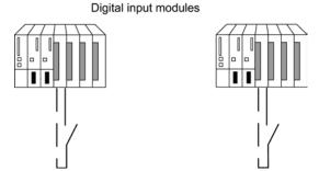
Figure 13-8 Fault-tolerant digital input modules in 1-out-of-2 configuration with two encoders
