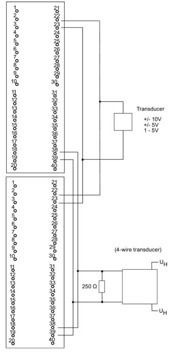
Figure E-27 Example of an interconnection with SM 331; Al 8 x 16 Bit
