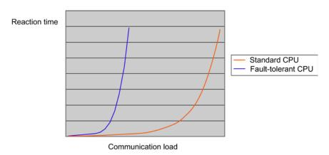
Figure 14-21 Communication load as a variable of response time (basic profile)
