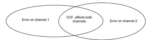
Figure A-3 Common Cause Failure (CCF)
