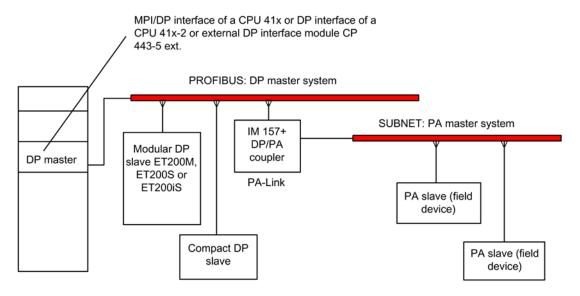
Figure B-1 Overview: System structure for system modifications during operation
