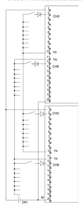
Figure E-5 Example of an interconnection with SM 321; DI 16 x DC 24V
