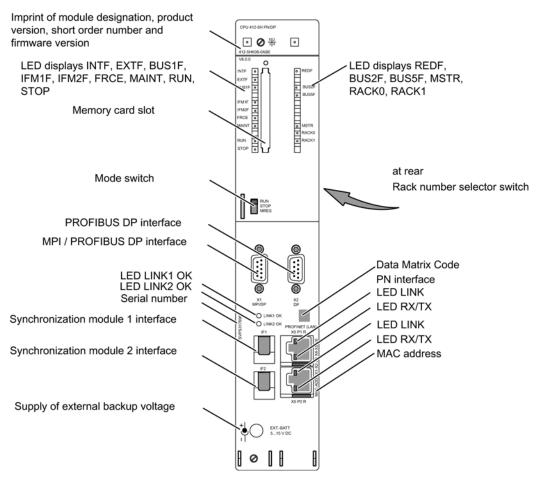
Figure 5-1 Arrangement of the control and display elements on CPU 41x-5H PN/DP
