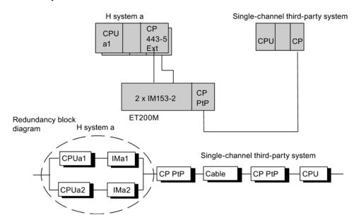
Figure 14-11 Example of connecting a fault-tolerant system to a single-channel third-party system using switched PROFIBUS DP
