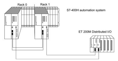
Figure 13-1 Single-channel switched distributed I/O configuration at the PROFIBUS DP interface
