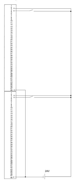
Figure E-12 Example of an interconnection with SM 421; DI 32 x 24 V
