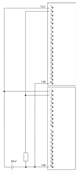
Figure E-19 Example of an interconnection with SM 322; DO 8 x DC 24 V/0.5 A
