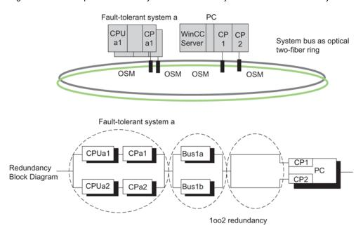
Figure 14-19 Example of redundancy with a fault-tolerant system, redundant bus system, and CP redundancy on PC.
