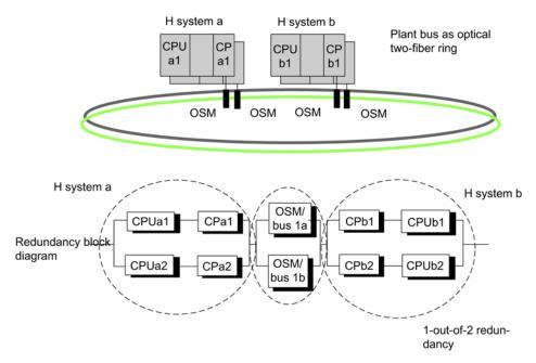
Figure 14-14 Example of redundancy with fault-tolerant system and redundant ring
