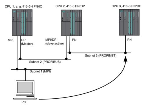
Figure 14-2 S7 routing gateways: MPI - DP - PROFINET
