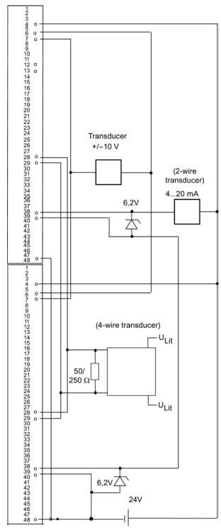
Figure E-34 Example of an interconnection with SM 431; Al 16 x 16 Bit
