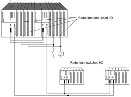
Figure 13-13 Redundant one-sided and switched I/O
