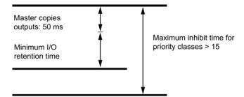
Figure 12-5 Correlation between the minimum I/O retention time and the maximum inhibit time for priority classes > 15
