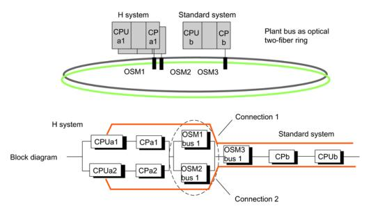
Figure 14-9 Example of linking of standard and fault-tolerant systems in a redundant ring
