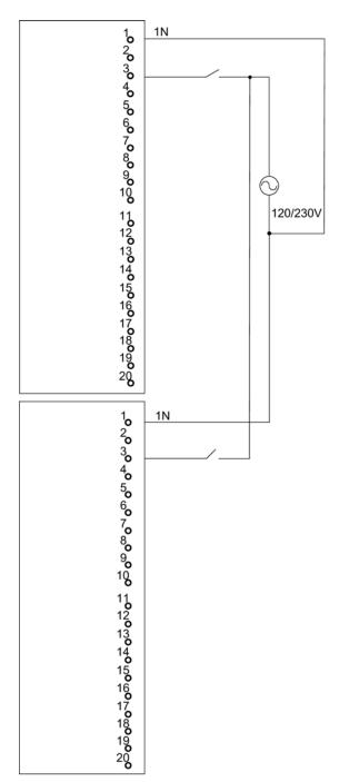
Figure E-4 Example of an interconnection with SM 321; DI 8 x AC 120/230 V
