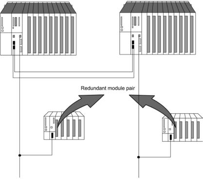
Figure 13-4 Redundant I/O in the one-sided DP slave
