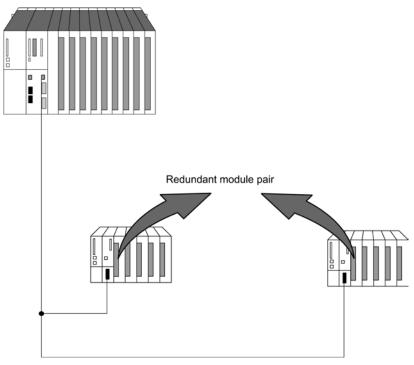
Figure 13-6 Redundant I/O in stand-alone mode
