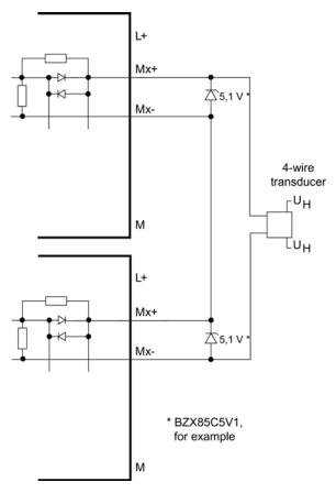
Figure E-30 Interconnection example 1 SM 331; Al 8 x 0/4...20mA HART
