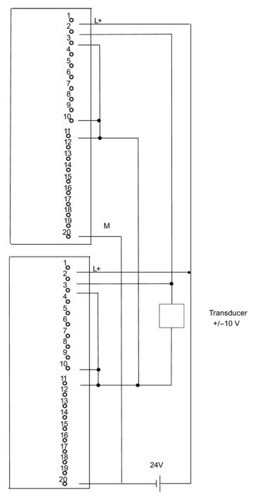
Figure E-26 Example of an interconnection with SM 331; Al 8 x 12 Bit
