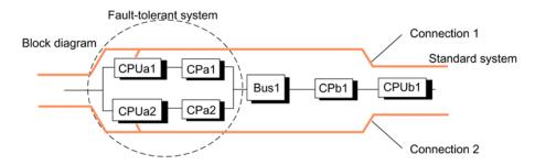
Figure 14-7 Example of linking standard and fault-tolerant systems in a simple bus system
