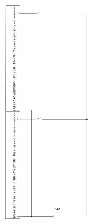
Figure E-13 Example of an interconnection with SM 421; DI 32 x 24 V
