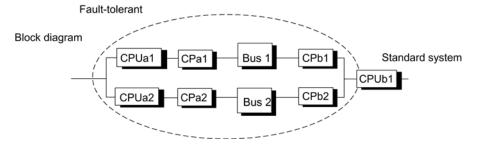
Figure 14-10 Example of redundancy with fault-tolerant systems and a redundant bus system with redundant standard connections
