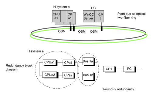
Figure 14-18 Example of redundancy with fault-tolerant system and redundant bus system
