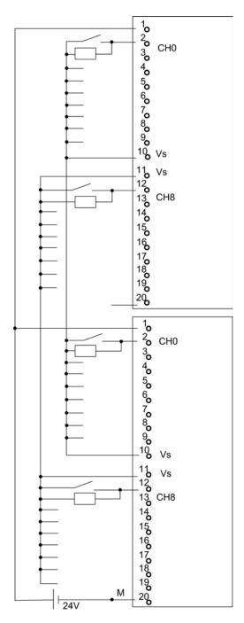
Figure E-6 Example of an interconnection with SM 321; DI 16 x DC 24V
