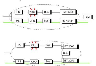
Figure 2-4 Example of redundancy in a 1-out-of-2 system with error
