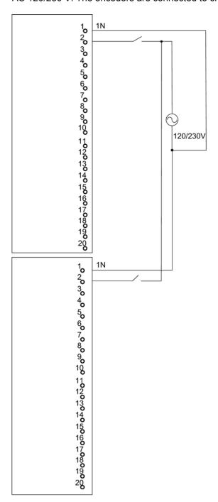
Figure E-3 Example of an interconnection with SM 321; DI 16 x AC 120/230 V
