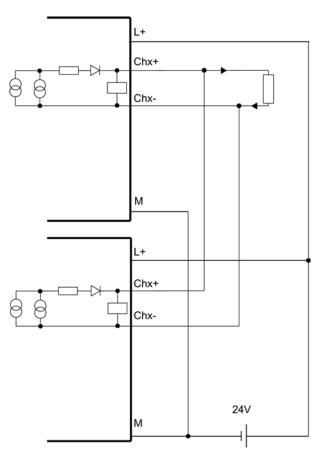
Figure E-33 Interconnection example 3 SM 332; AO 8 x 0/4...20mA HART
