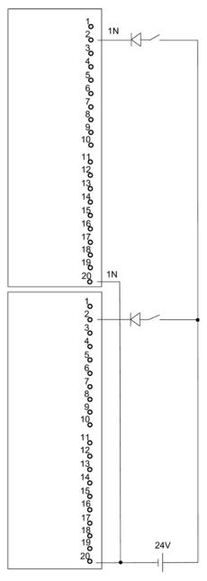
Figure E-1 Example of an interconnection with SM 321; DI 16 x DC 24 V
