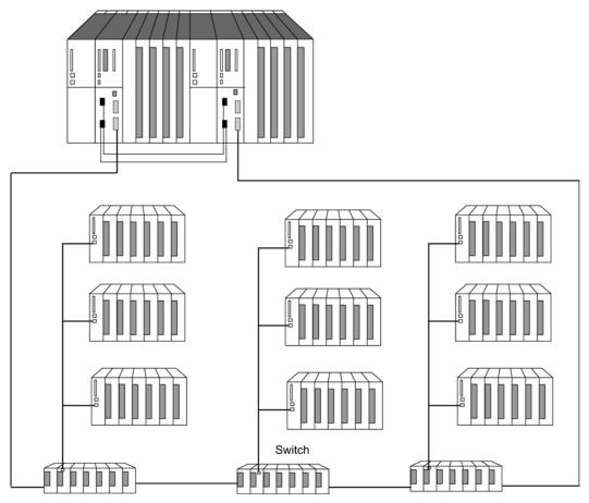
Figure 8-5 PN/IO with system redundancy
