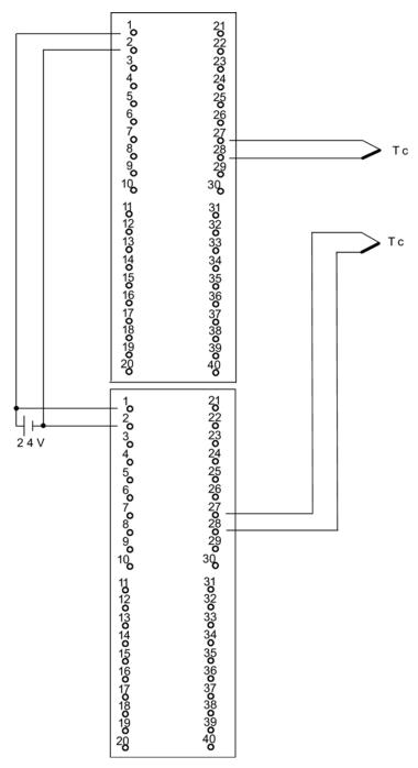
Figure E-29 Example of an interconnection AI 6xTC 16Bit iso
