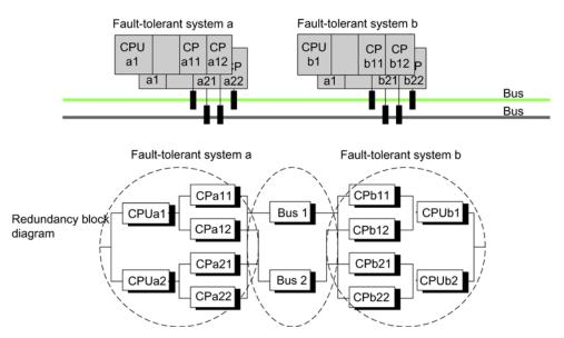
Figure 14-16 Example of fault-tolerant system with additional CP redundancy
