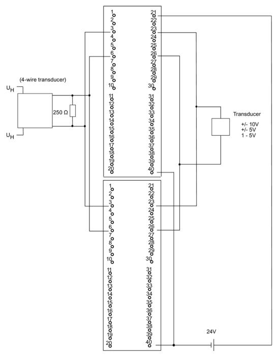
Figure E-28 Example of an interconnection with SM 331; Al 8 x 16 Bit
