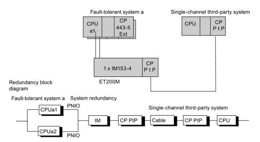
Figure 14-12 Example of connecting a fault-tolerant system to a single-channel third-party system using PROFINET IO with system redundancy
