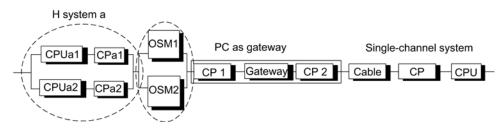
Figure 14-13 Example of linking a fault-tolerant system to a single-channel third-party system
