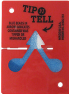
Figure 3-4 Tilt indicator tripped
