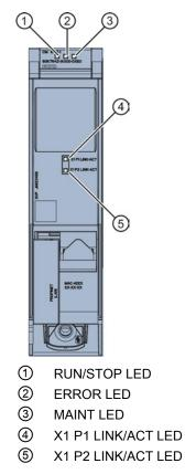
Figure 3-1 LED display of the CM 1542-1 (without front cover)
