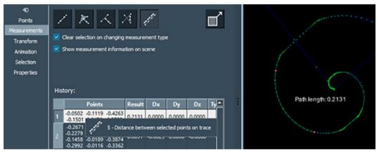
Figure 10-7 Measure the point distance on the tool path
