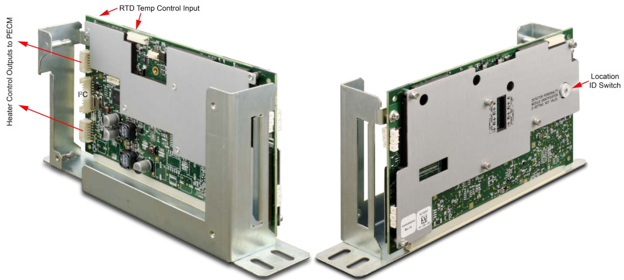
Figure 2-29 Temperature Control DPM Connections
