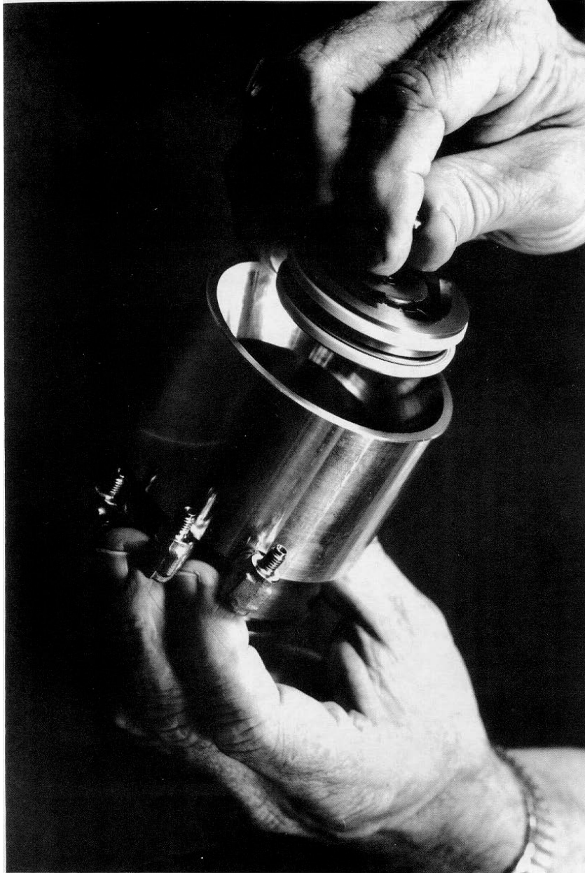
Figure 4-39: Inserting Piston Assembly (15 and 18) into Base (16)
