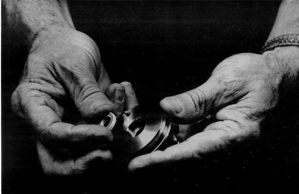
Figure 4-37: Installing Bal-Seal (20) in Piston Groove (18)
