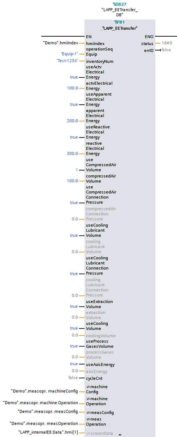
Figure 2-59 LAPP\_EETransfer block
