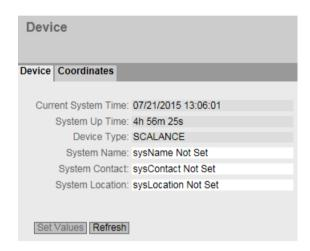
The boxes "Current System Time", "System Up Time" and "Device Type" cannot be changed.
