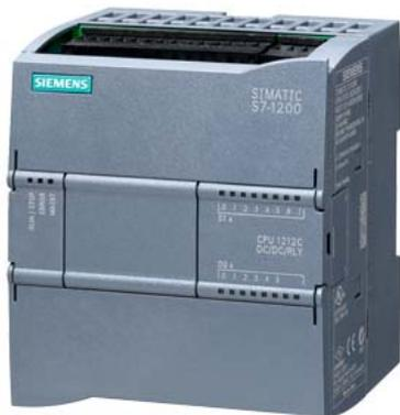
SIMATIC S7-1200, CPU 1212C, compact CPU, DC/DC/relay, onboard I/O: 8 DI 24 V DC; 6 DO relay 2 A; 2 AI 0-10 V DC, power supply: DC 20.4-28.8 V DC, program/data memory 100 KB
